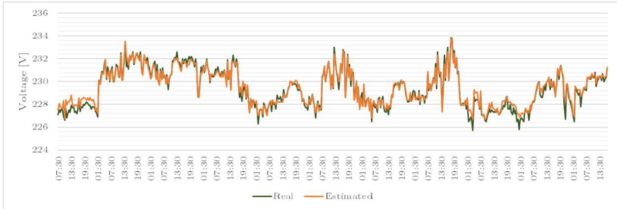
Figure 3-5: Comparison between estimated and real voltage values for one smart meter (id: L2 [37341193]) connected to phase b, over the period of 10 days.
